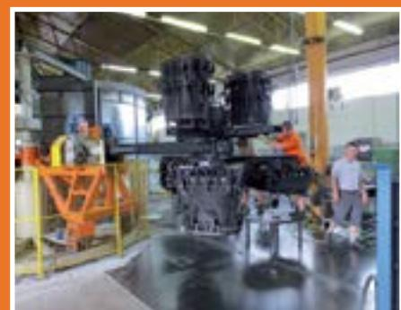
Rotational shaping of plastic masses is a production method used for manufacturing plastic products. It differs from all other process methods by the fact that the heating, melting, shaping and cooling stages take place only after we insert the polymer into the mould and that external pressure is not needed during the shaping process.
