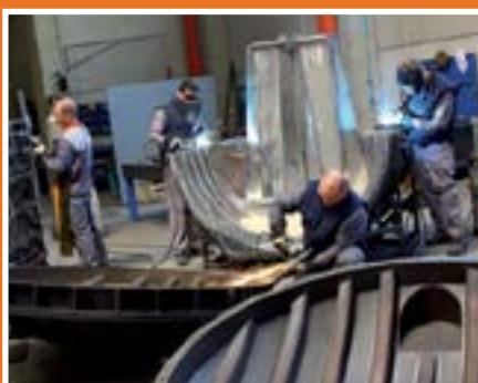
We have mastered all the necessary technology for manufacturing high-quality moulds for rotational moulding. The tool manufacturing process encompasses modelling, technical documentation, manufacturing a sheet metal mould, or a steel or aluminium mould using CNC milling and sandblasting.
