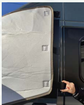
Magnet fastening for optimal shutter tension without any risk to the bodywork
